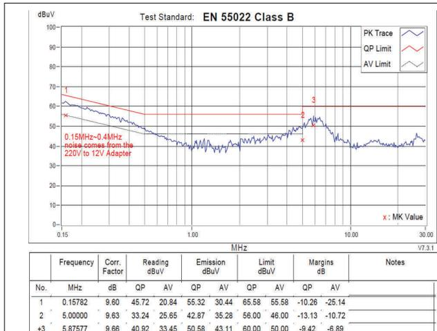
**Figure 8-5. Conducted Emission with Ferrite Bead Filter - Line**
