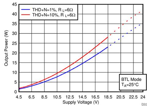
NOTE: Dashed lines represent thermally limited region for the continuous output power.
