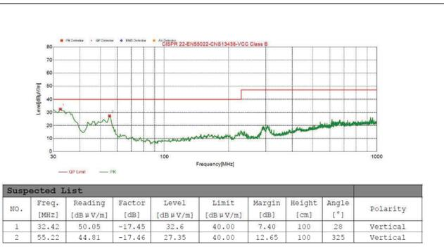
**Figure 8-8. Radiated Emission with Ferrite Bead Filter - Vertical**
