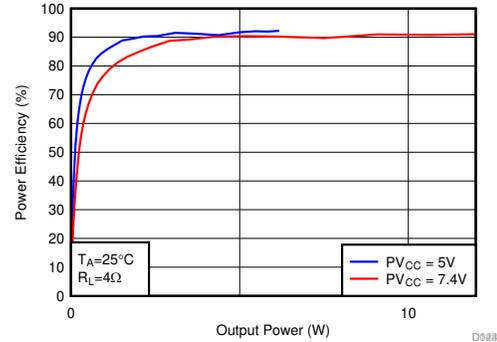
PVDD = 5V/7.4V      Ferrite Bead +      Spread Spectrum
