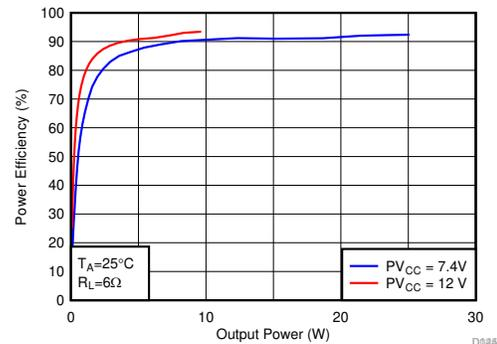
PVDD = 7.4V/12V      Ferrite Bead +      Spread Spectrum
