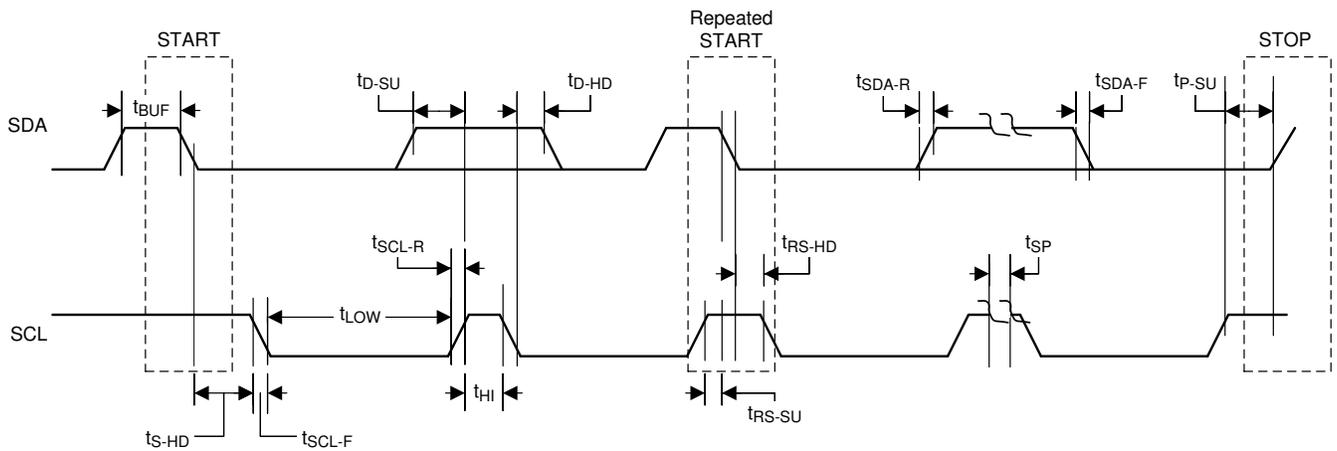
Figure 7-2. I<sup>2</sup>C Communication Port Timing Diagram
