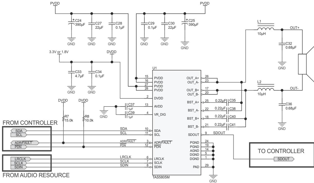
Figure 8-9. Mono (PBTl) System Application Schematic
