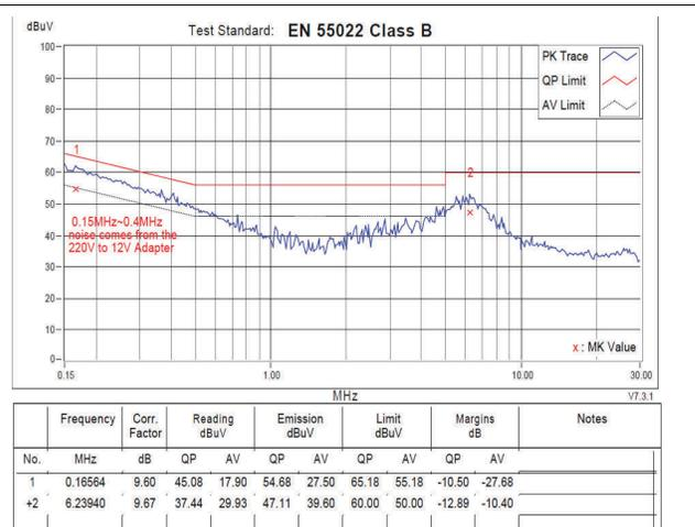
**Figure 8-6. Conducted Emission with Ferrite Bead Filter - Neutral**
