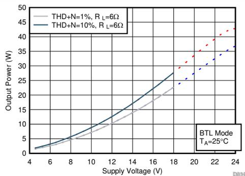
NOTE: Dashed lines represent thermally limited region for the continuous output power.
