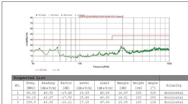
**Figure 8-7. Radiated Emission with Ferrite Bead Filter - Horizontal**
